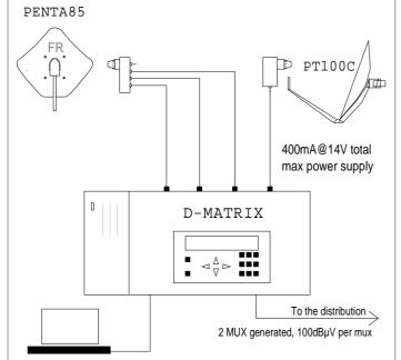
The D-MATRIX-4S headend can tune up to four different SAT trasponders, decrypt the programs (through CAMs & Smart-Cards - NOT INCLUDED) and generate two separate fullband RF Digital Multiplex (DVB-T or DVB-C), 100dBµV each.
